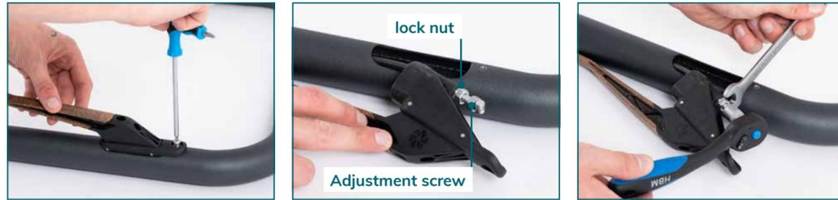
First remove the brake bar as described in point 5.5.3, if it is mounted.
