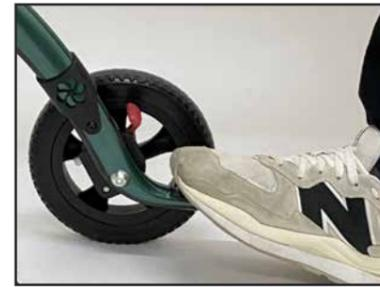
The tipping aid is located behind the rear wheels. Step on the tipping aid with one foot and pull the rollator slightly towards you using the handles. The front wheels are now in the air. This way you overcome thresholds and curbs.
