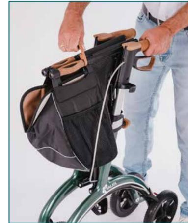
Open the brown hook to unlock the folding mechanism.
