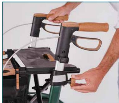
Open the hand screws on the handlebars. On the inside of the support bars you will find a height scale that makes it easier to adjust the left and right handlebars to the same height.
