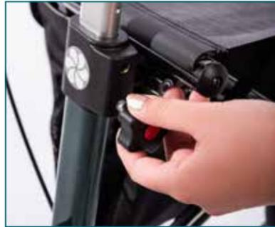
Open the hand screws on the handlebars. On the inside of the support bars you will find a height scale that makes it easier to adjust the left and right handlebars to the same height.
