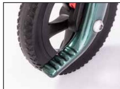
The tipping aid is located on the rear wheels. Step on the tilt lever with one foot and pull the rollator towards you gently by the handles. The walker will now tilt. This will help you overcome thresholds and curbs.
