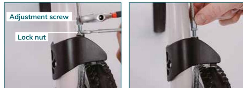
Loosen the lock nut with a size 8 open-end spanner and turn it completely upwards. Fix the adjustment screw at the same time.
